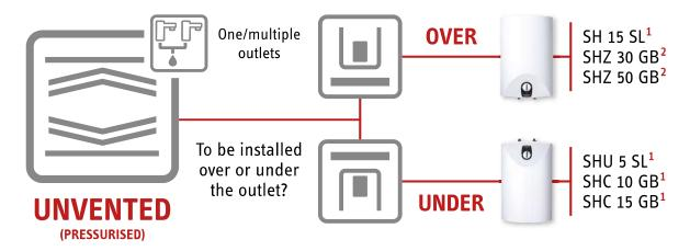
An additional unvented kit is needed if you do not have more than 2.0 m for the 5 litre, 2.8 m for the 10 litre, 4.2 m for the 15 litre 15mm pipe length between heater and outlet. Unvented kit - 236701 for the 5 & 10 litre models & 236702 for the 15 litre model.
